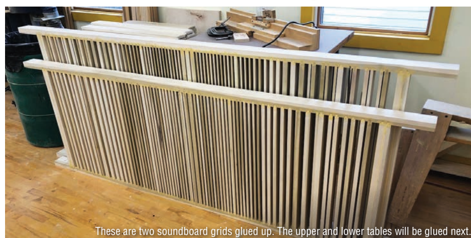
This is the 'grid', the heart of one of the slider soundboards. It is essentially a large frame with many bars that act as dividers or partitions between each note channel.
